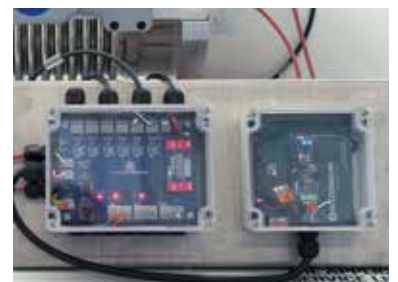
The measurement electronics and data transfer facility are applied externally especially for hot and insulated pipelines.
