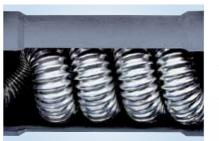
The heat exchanger consists of a compact, spiraled stainless steel corrugated hose in a high-quality plastic housing. On the heating-side, two or four threaded nipples are embedded in the housing. The pool water pipework connection is via a PVC-glued joint. In addition, all housings have a thermowell for incorporating an electrical temperature sensor.
